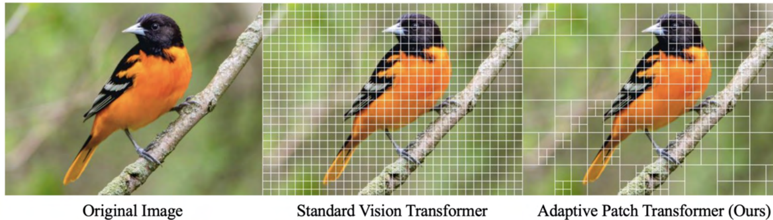
Figure 1: Adaptive Patch Sizing. We present APT, Adaptive Patch Transformers, which significantly accelerate vision transformer training and inference by patchifying images based on their content. Complex regions receive more, smaller tokens, while simpler, homogeneous regions receive fewer.
