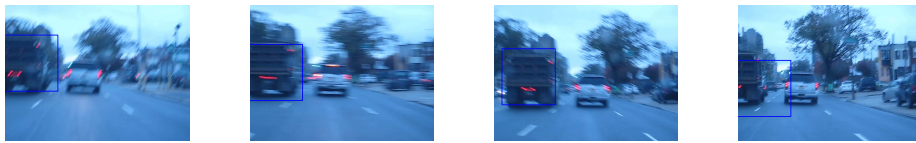
(d) Tracking the transporter on the left side works well, even in case of occlusions as in the last image.
