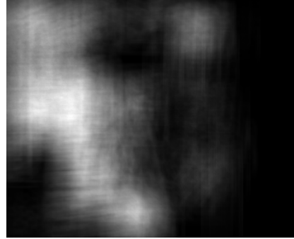
Figure 8: The left part of the image has much more points with high gradient magnitude and thus the points in this half get much more votes than the points in the right half where the ROI actually is in the shadow.
