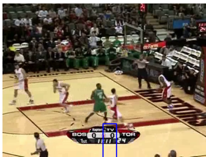
Figure 9: The player movement from the first to the second frame changes the gradient orientations of the pixels so much that the Generalized Hough Transform can not find the player anymore.
