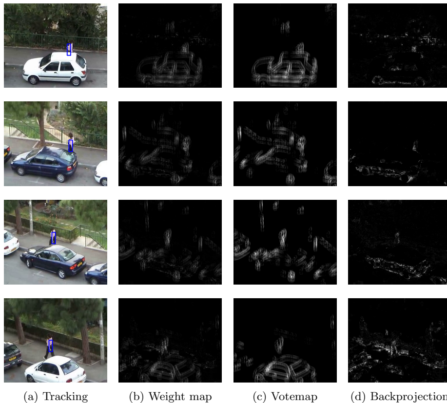
Figure 11: Combining histogram-based tracking (d) and the Generalized Hough Transform (c) using a weighted sum of the two (b) results in consistent tracking of the woman across the entire video (a).
